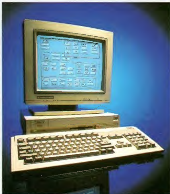
The A3000 - a nice machine, although a bit fussy. Its main advantage as a starting point is that it is cheap and has Zorro III slots.
